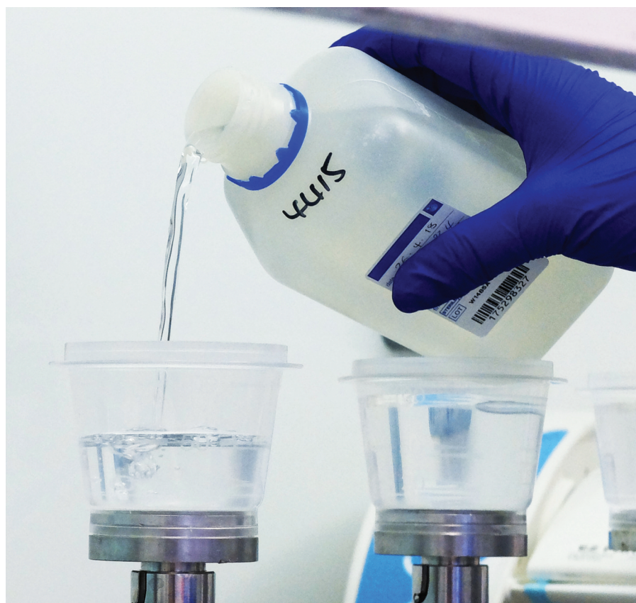
The current method of testing Mycobacteria is membrane filtration and 28-day incubation.
